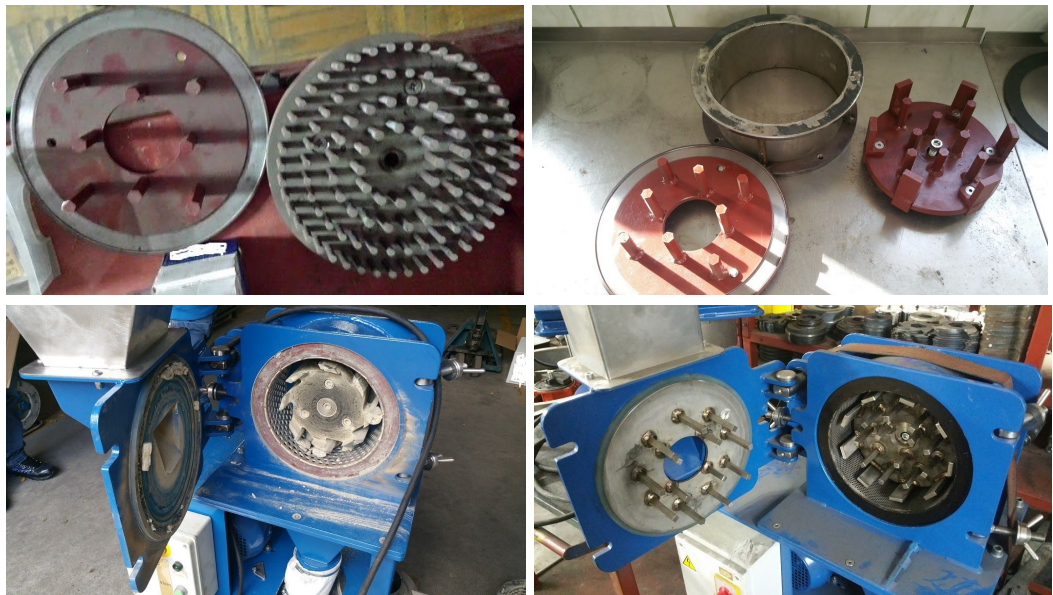
RM rotor / pin solutions (depending on application)
